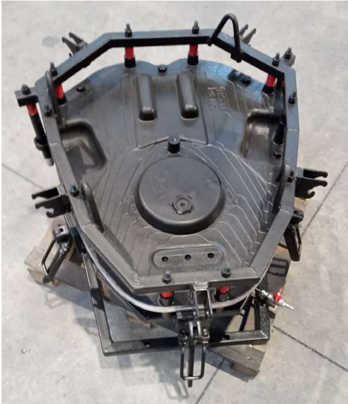
> Moulds for rotational moulding of the three structure components.
