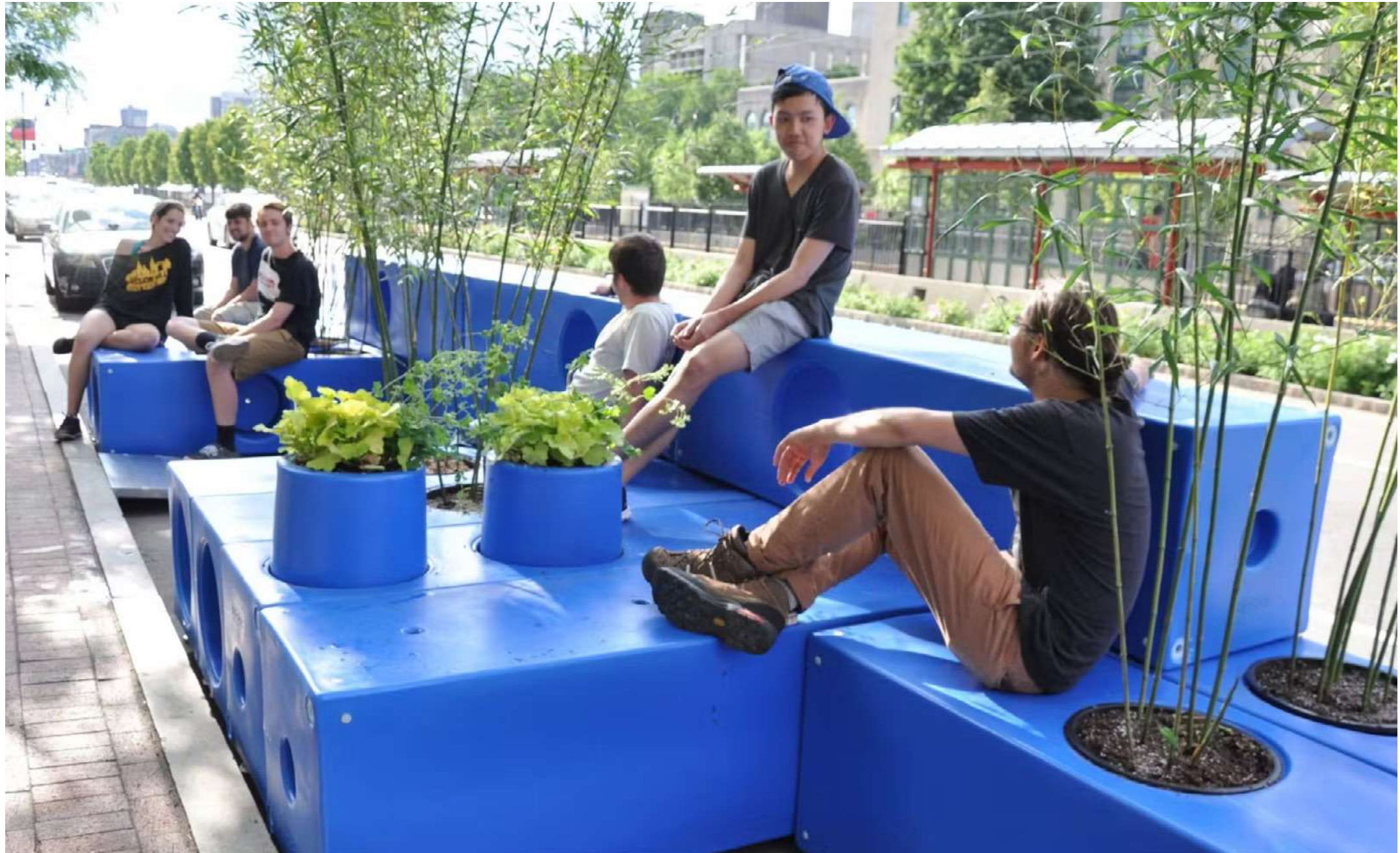
> The Ad-bloc can be configured in many ways and blocks can be joined together using a plug as an interlocking mechanism.
