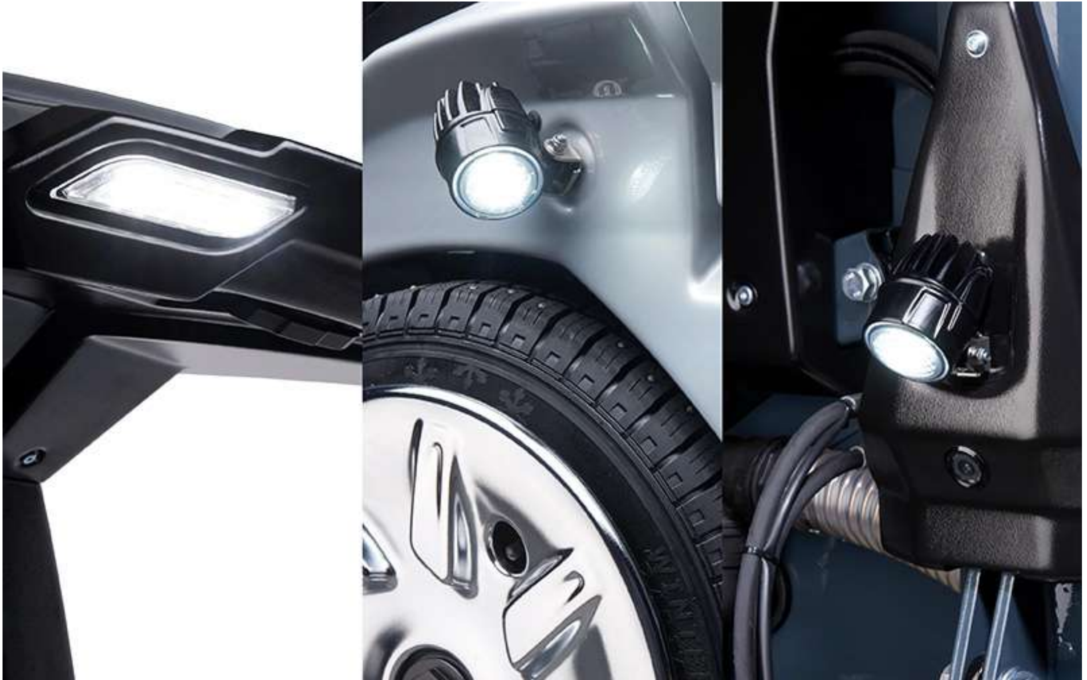
> Front and working lights have been designed to be integrated into the moulded components.
