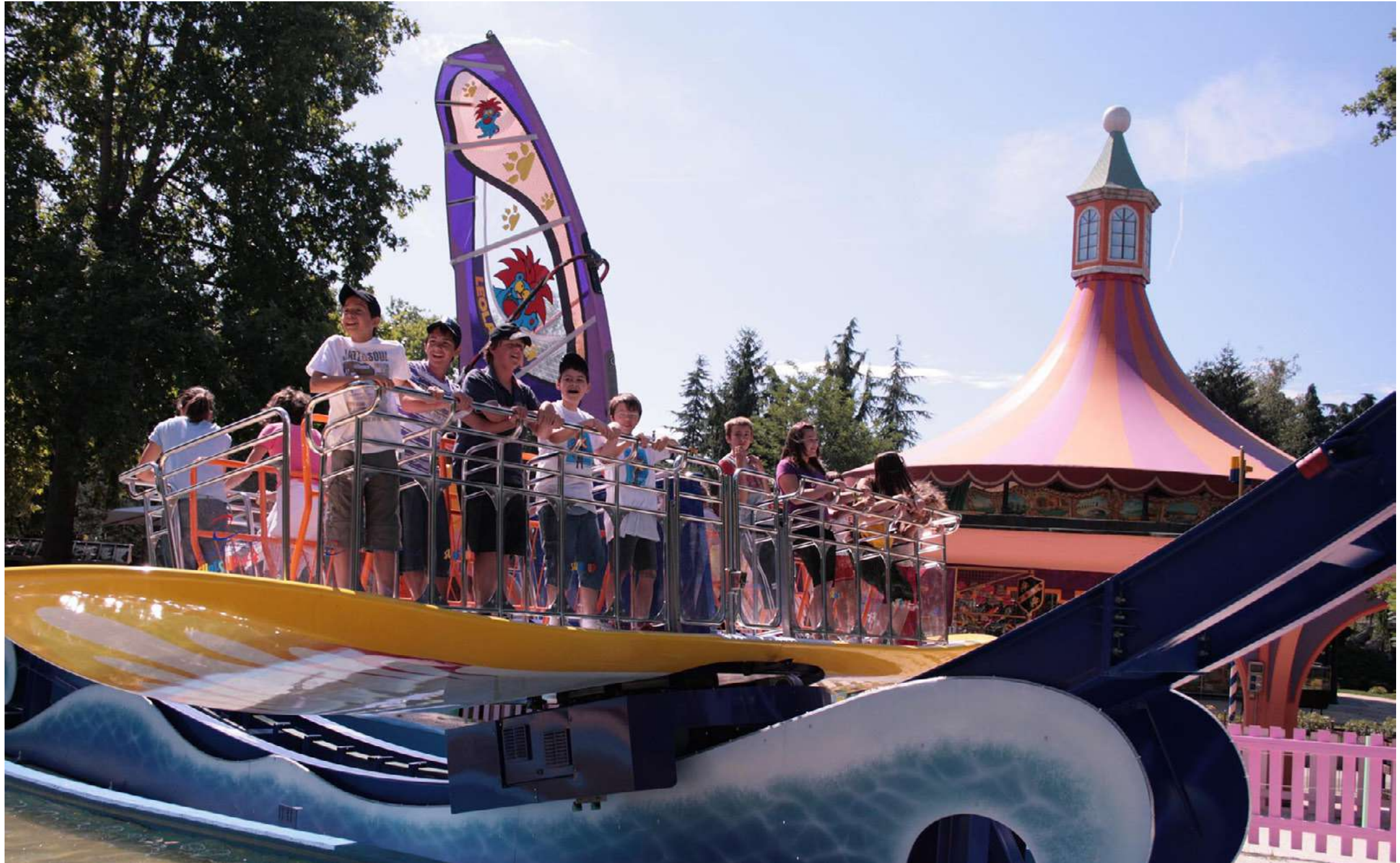
> The tilting base is made of steel and covered with a fiberglass cover.
