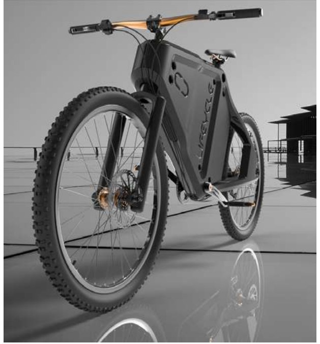
> A hollow rotomoulded twin shell frame
