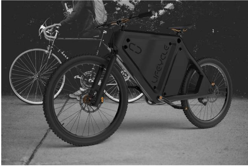
> A hollow rotomoulded twin shell frame
