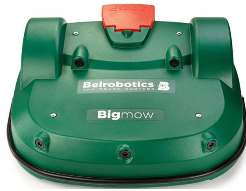
> Bigmow is fitted with sonars deactivating its cutting system if it detects an obstacle.
