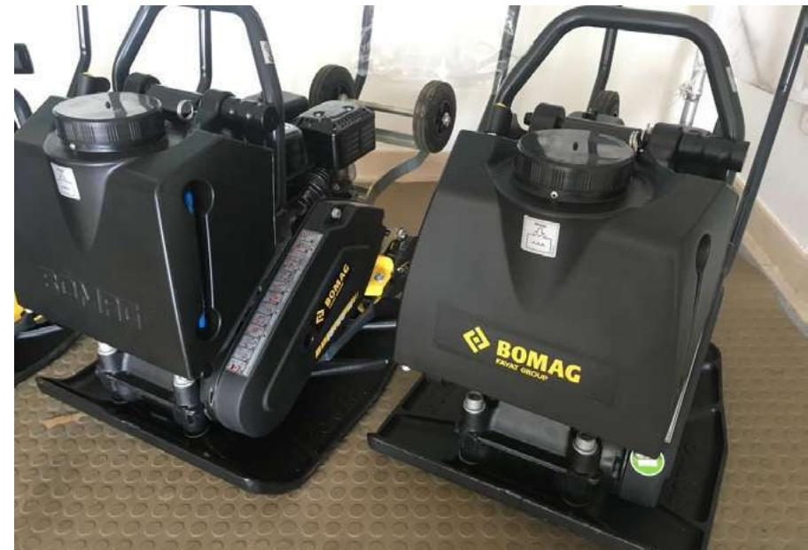
> The hinged guide handle is mounted on effective "silentblock" rubber mounts which reduce hand/arm vibrations to the minimum.
