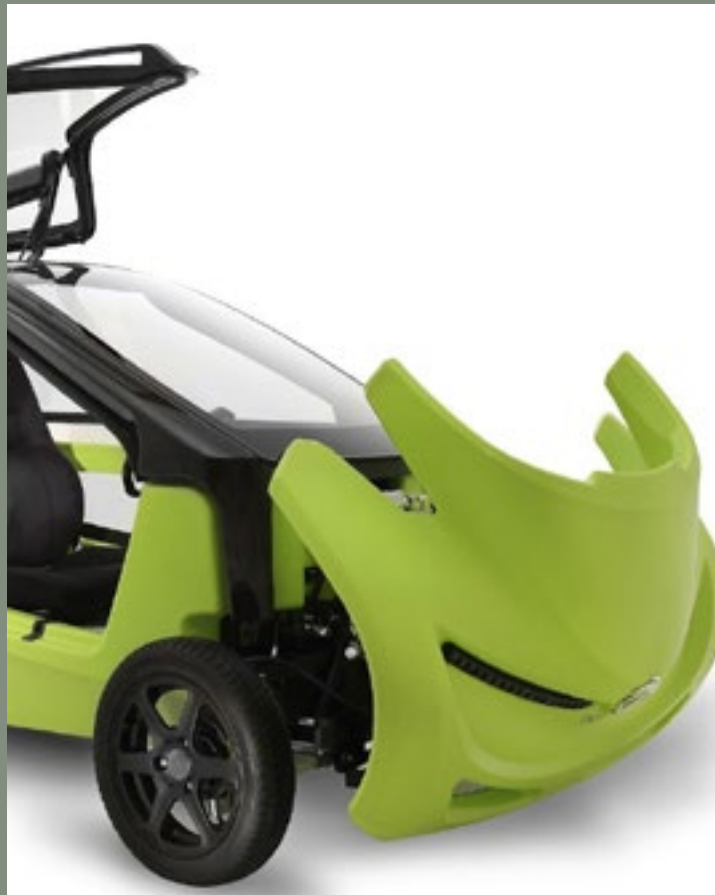
Total Car, electric city car with some body parts rotomoulded using a modified polyethylene alloy and PLA. 2011
