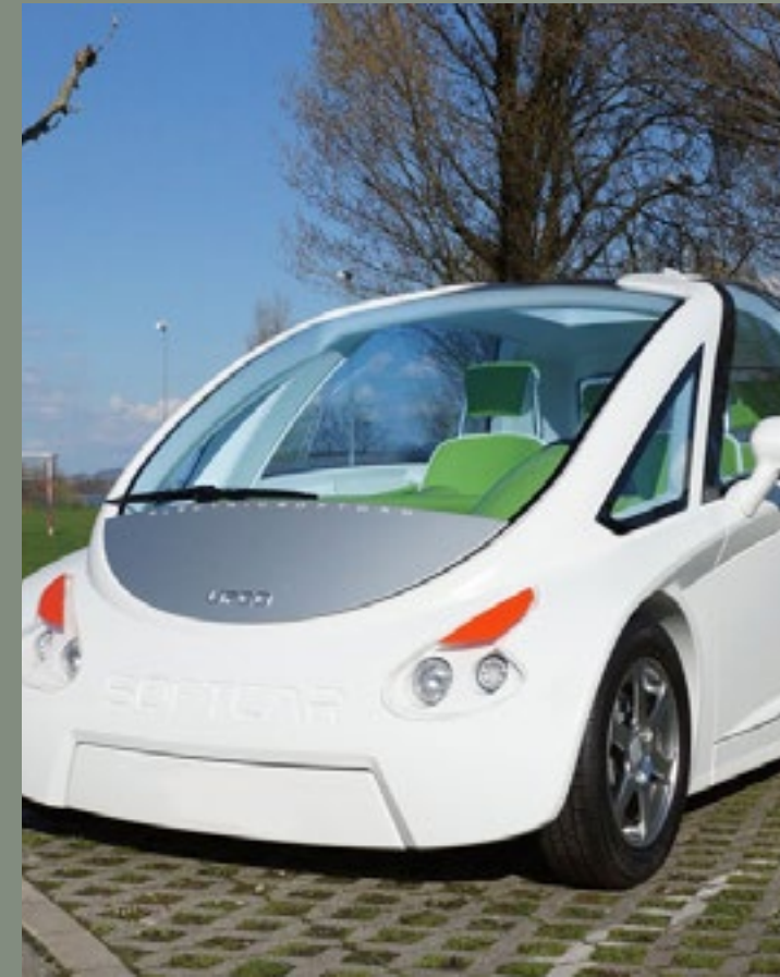
SoftcarUpgo is based on an aluminium chassis covered with a recyclable thermoplastic. 2015
