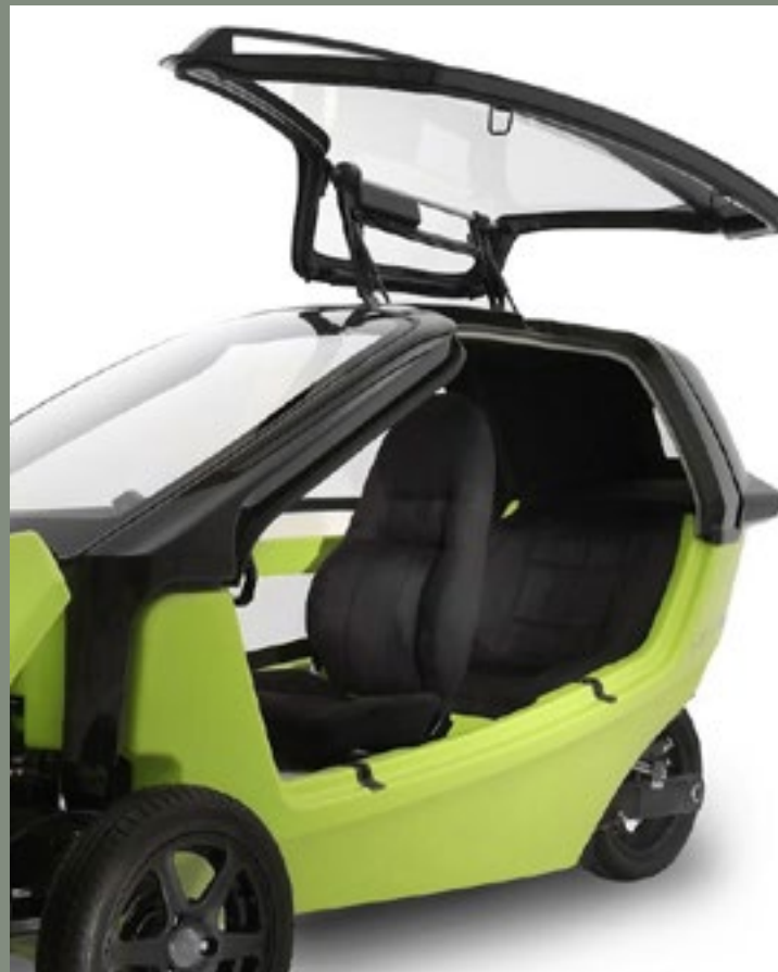
Total Car, electric city car with some body parts rotomoulded using a modified polyethylene alloy and PLA. 2011
