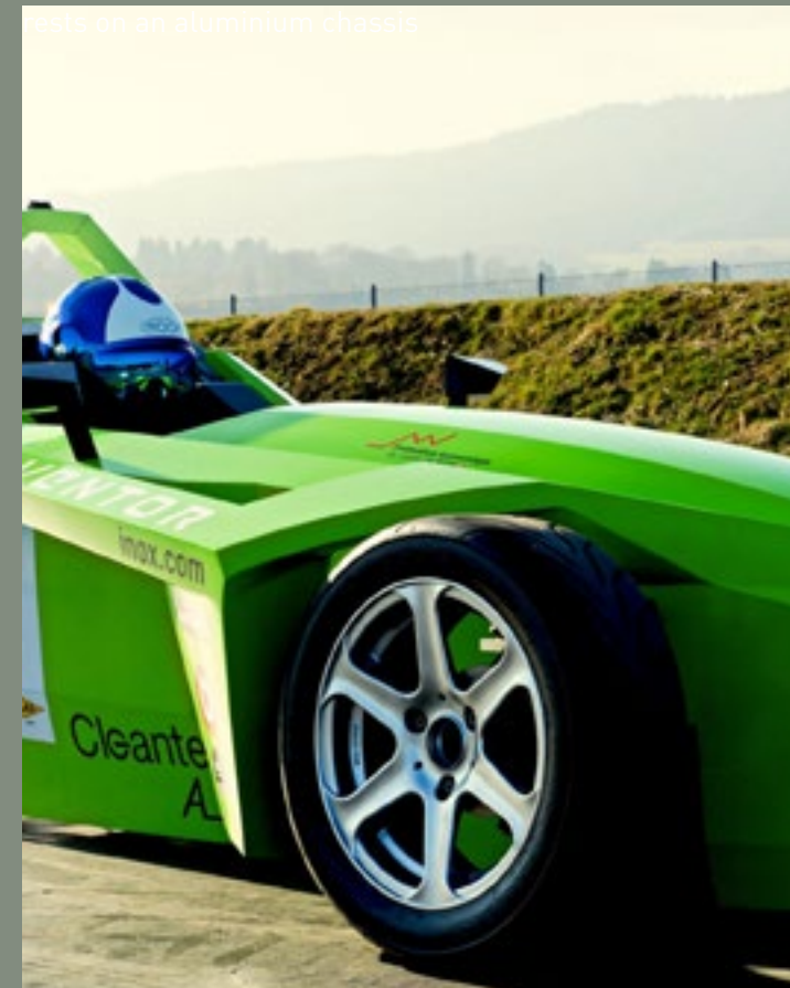
Totally recyclable, Aventor's bodywork is made from bio-polymers and rests on an aluminium chassis. 2014
