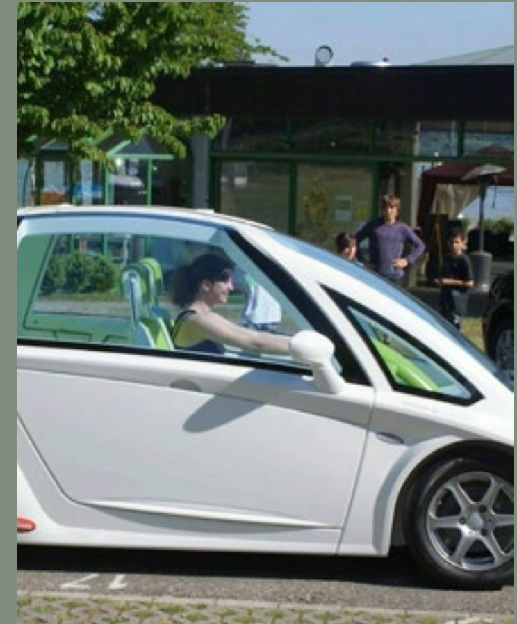
SoftcarUpgo is based on an aluminium chassis covered with a recyclable thermoplastic. 2015
