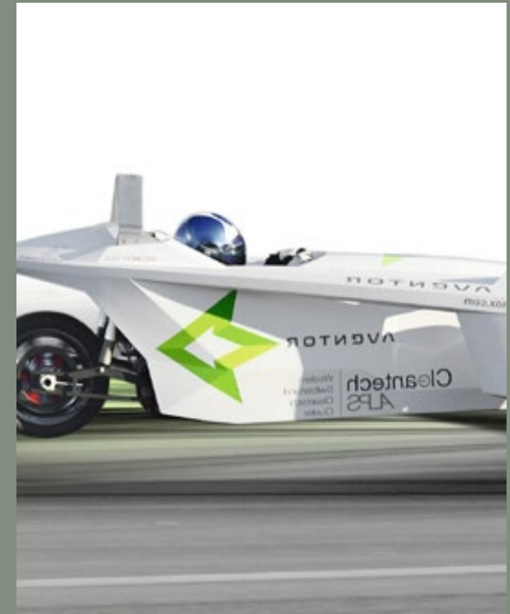
Totally recyclable, Aventor's bodywork is made from bio-polymers and rests on an aluminium chassis. 2014
