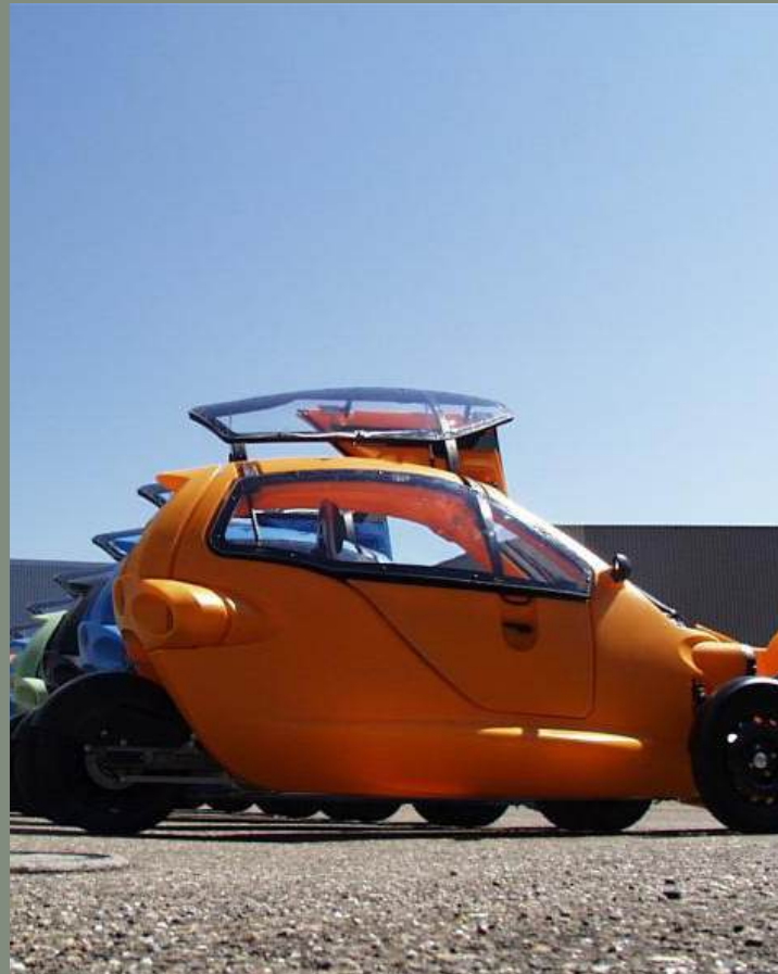
Cree SAM, is a zero emission battery electric vehicle. It's a three-wheel car, with two seats in a tandem arrangement. 2011
