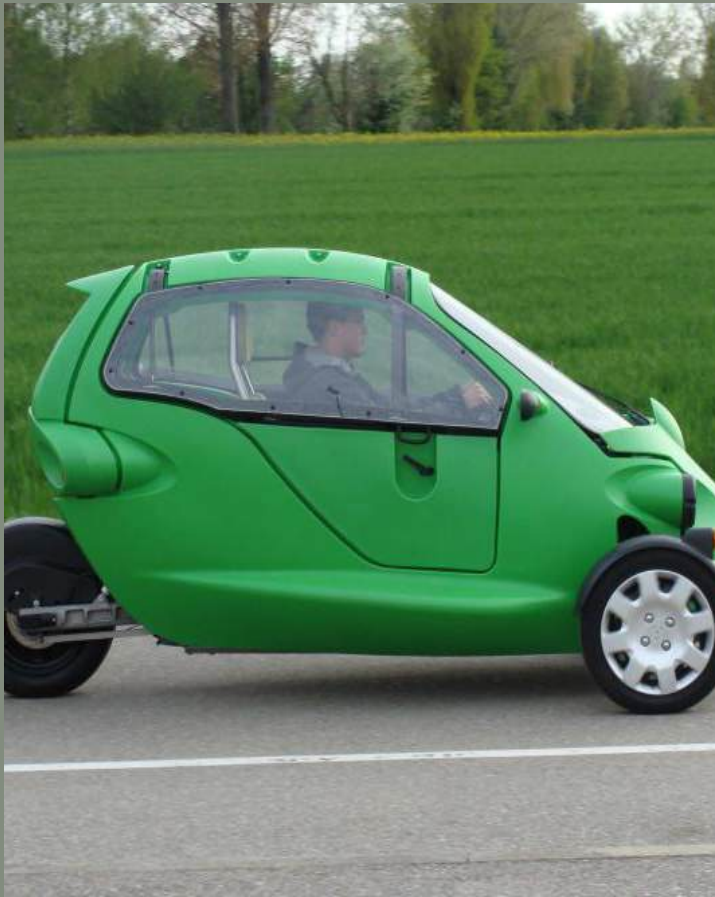
Cree SAM, is a zero emission battery electric vehicle. It's a three-wheel car, with two seats in a tandem arrangement. 2011
