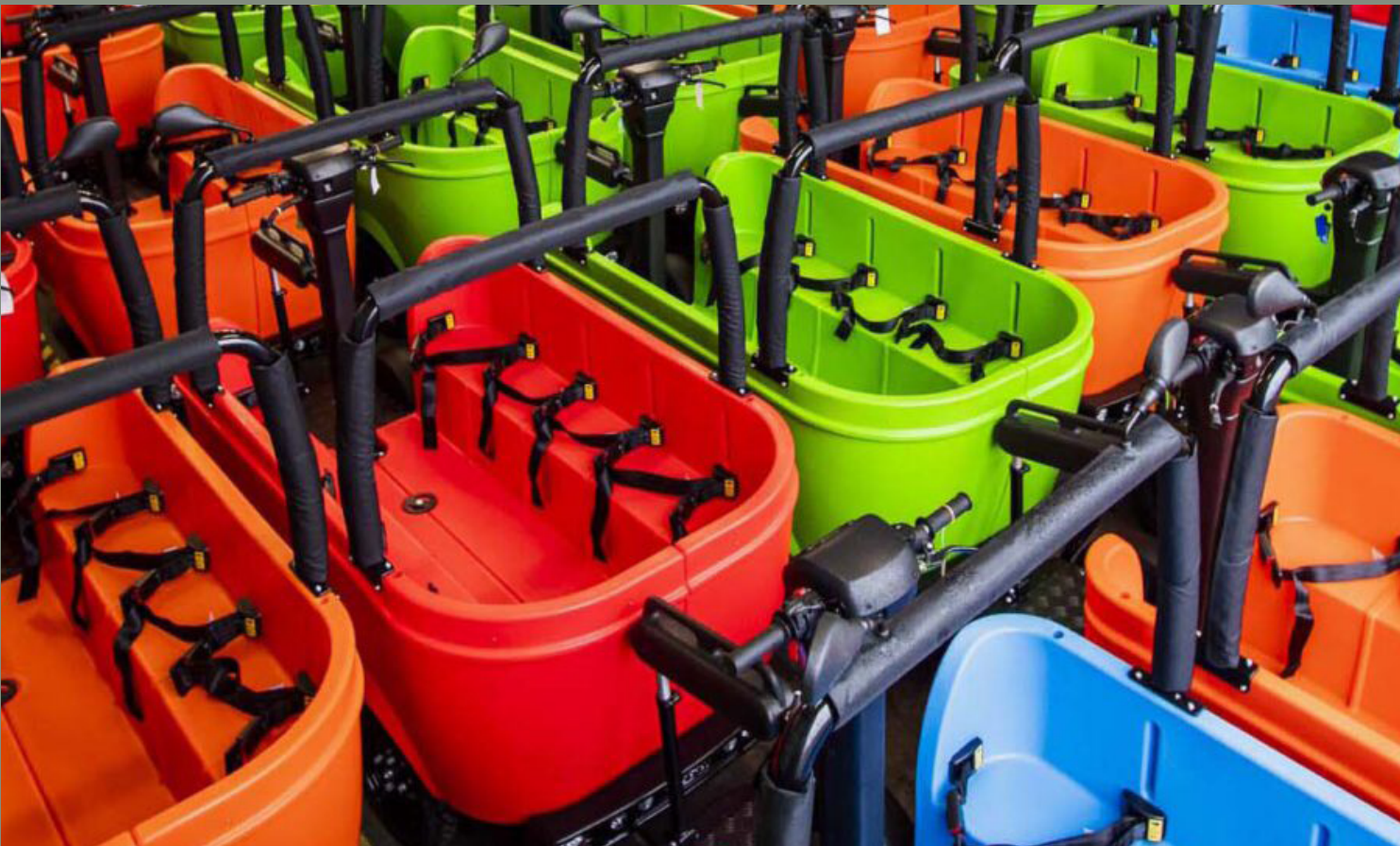
The rotomolded compartment is equipped with seat belts and can carry up to ten children.
