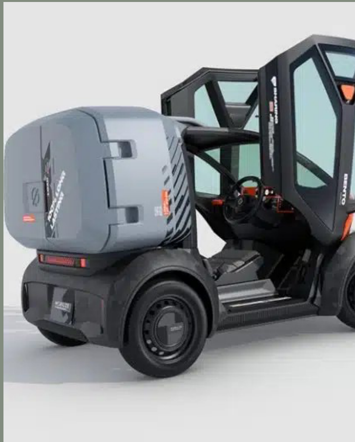
The rotomoulded container on the back can be customised with graphics and adhesive elements.
