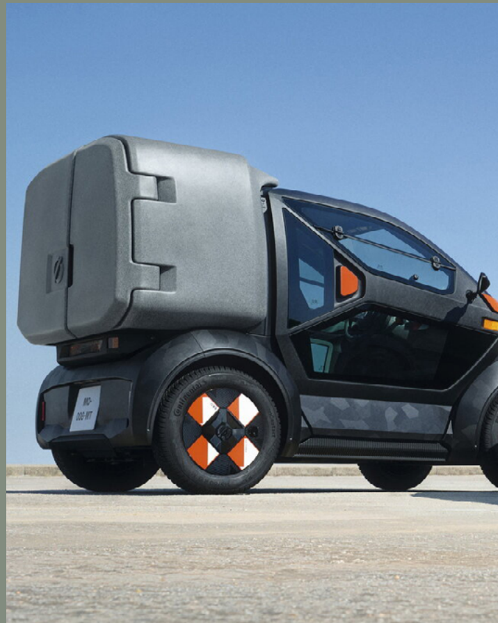
The rotomoulded container on the back can be customised with graphics and adhesive elements.
