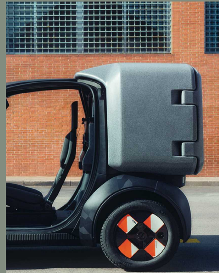
Sturdy moulded hinges allow the two rear doors to be opened easily.
